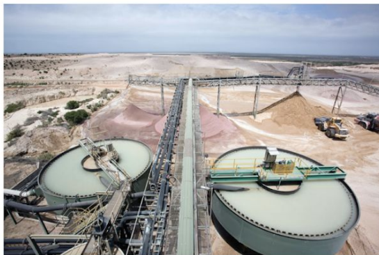
Process water recycling and garnet slime extraction unit in the wet plant. Piles of pinkish garnet raw concentrate (left) and sand (right), which is trucked back to the mine for backfill.
